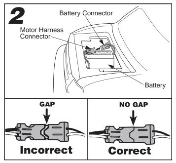
Plug the battery and motor harness connectors together. Push firmly to make sure the two connectors are completely joined.
